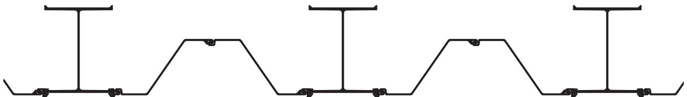
**HZ 575 king piles / AZ 18 intermediary sheet pile combined wall**
